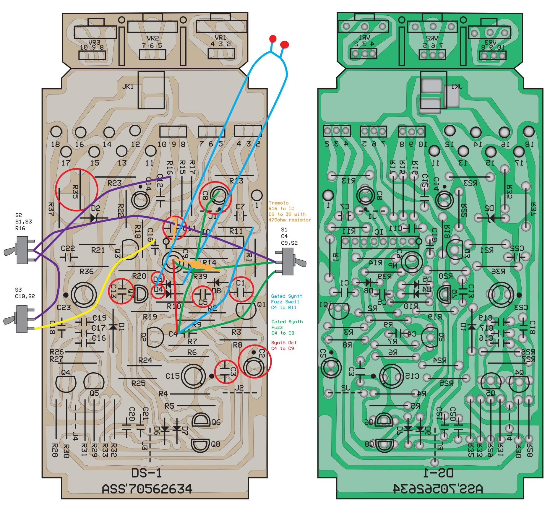
JHS Synth Mod C1, C5- .1u Input caps, raise value to allow broader range of signal into the clipping stage
